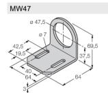
69452 Mounting bracket; material: Steel plate, galvanized
