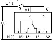
For the functions E, W, H, I, P, and B the terminal B1 can be connected with A1 and the device will start with the power supply.
