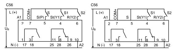
Start up with bridge between 5 and 7. Considering of precision reasons it is only recommended by using longer times.
