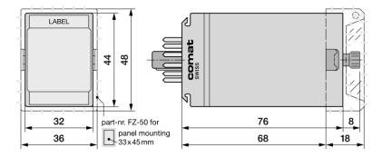
Noryl SE1, Lexan EXL 9330 (UL 94V-1) IP40 80 g Socket 11-pole (IEC 67-1-18a), (retaining clip or front mounting set) IEC571 >> 20g
