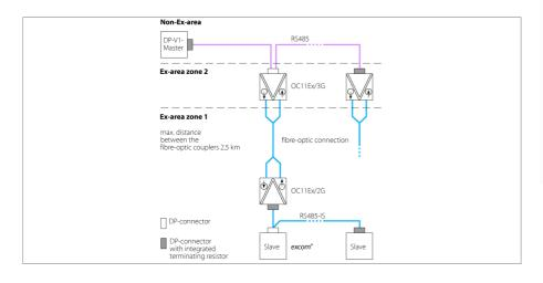
The optocoupler OC11Ex/2G.2 converts the PROFIBUS-DP signals on copper cables into optical signals. The bus signals can therefore be transmitted from the safe area to the Ex area over long distances without potential or interference. When using fiber-optic cables, the maximum baud range is 2500 m for OM1 (62.5/125- $\mu$ m) cables and 1500 m for OM2 (50/125- $\mu$ m) cables.
