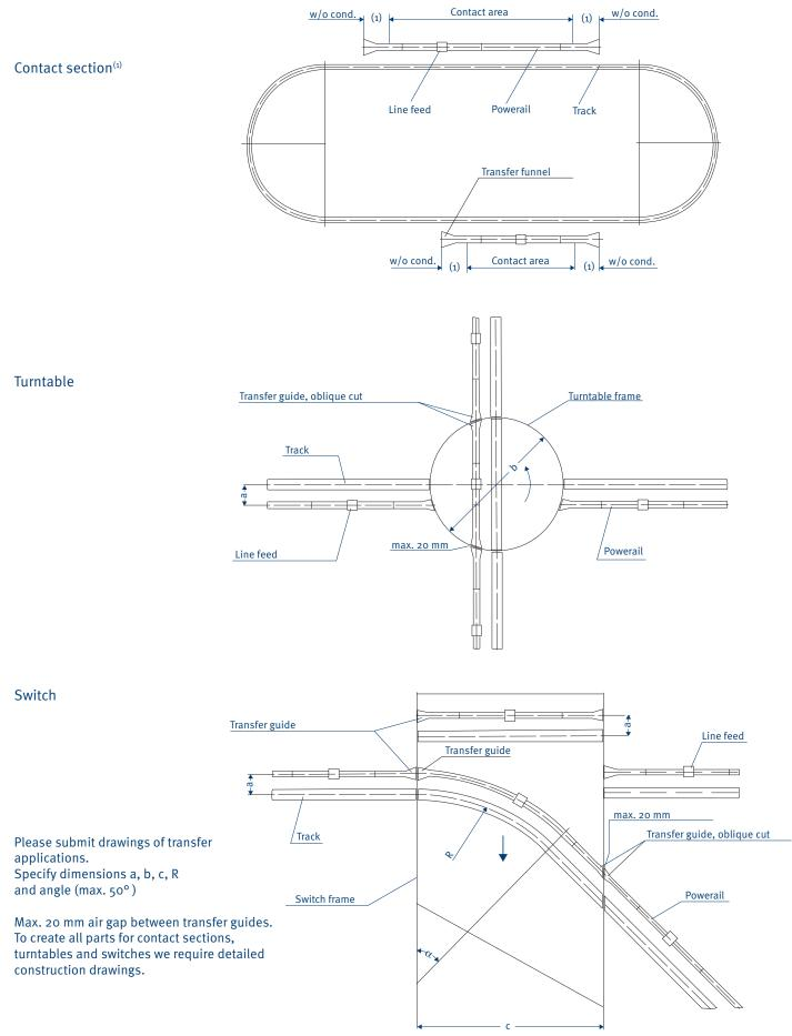
(1) Contact sections must not be activated before collectors are fully engaged.
