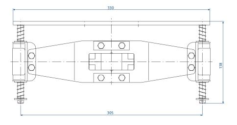
max. horizontal offset =10 mm max. vertical offset = 10 mm
