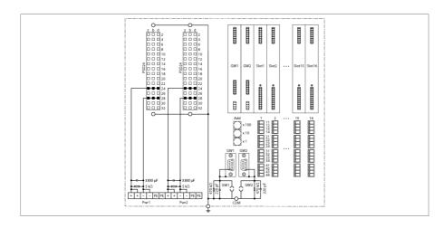
The MT16-2G module rack consists of a backplane, two PS-F24Ex mains filters and the actual rack system. It can accommodate 2 gateways, 2 power supply units as well as 16 I/O modules. Up to 128 binary inputs/outputs or 64 analog inputs/outputs resp. a mix of both can be connected to it. Two PS-F24Ex mains filters are mounted on the module rack. The mains filters filter the 24 VDC voltage and protect against induced interference in the supply cable.
