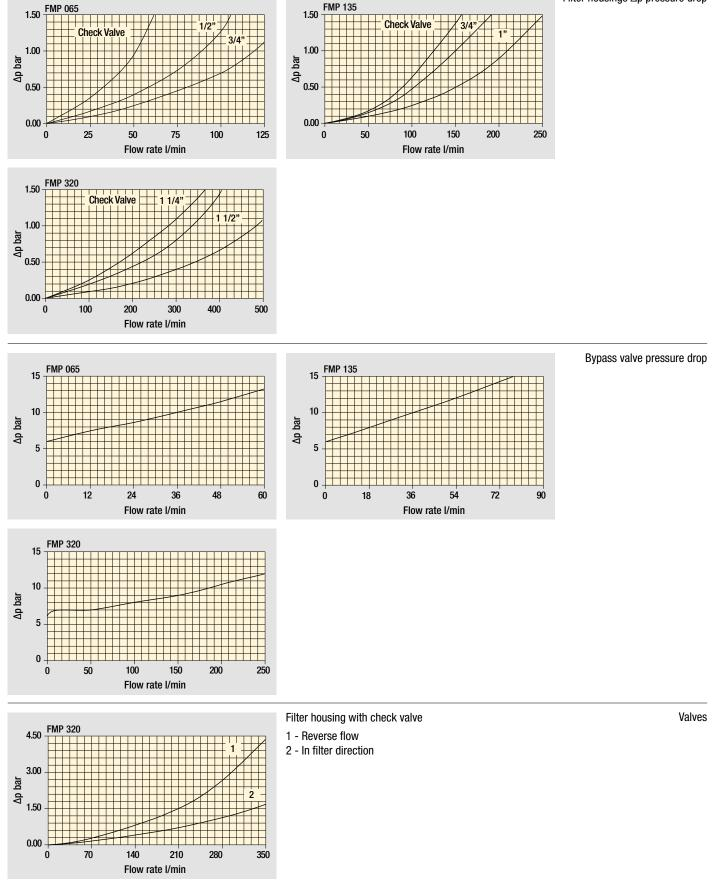
The curves are plotted using mineral oil with density of 0.86 kg/dm<sup>3</sup> in compliance with ISO 3968.  $\Delta p$  varies proportionally with density.
