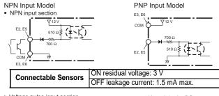
Note: A 2-wire DC sensor can also be connected. Check the ratings and characteristics tables, however, for the connection conditions.
