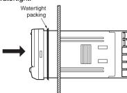
3. Insert the fixture into the grooves on the left and right sides of the rear case and push until it reaches the panel and is fixed in place.
