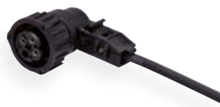
Ready-made cable Type FL33X33X 3 x 0,75 mm 2 with 4-pin bayonet ISO 15170 90° angle
