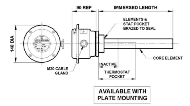
This range is recommended for applications where the equipment cannot be easily drained. Heat is transferred to the liquid by means of removable ceramic heating elements within a carrier tube to allow replacement without draining. Automatic control can be achieved by fitting a thermostat into the integral pocket. Sheath material available in stainless steel or mild steel. Rating up to 6kW.
