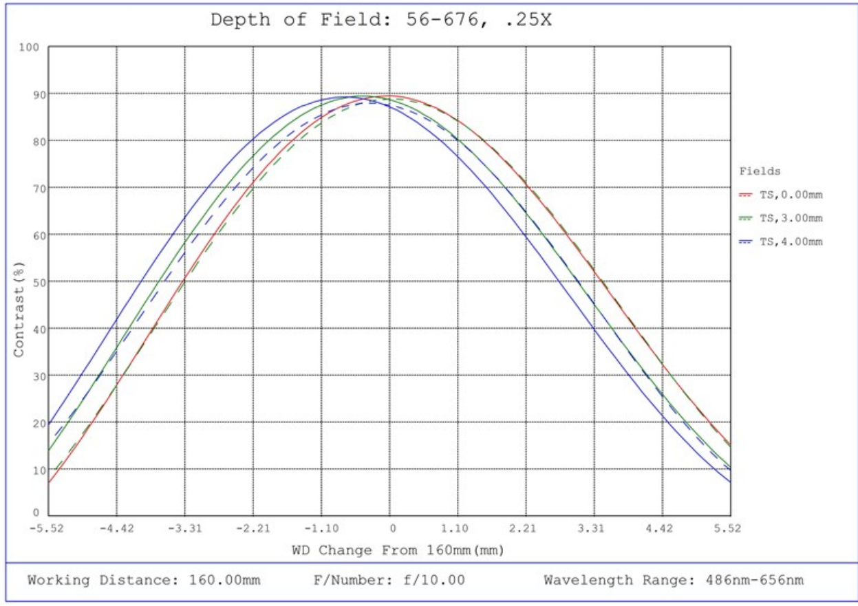
#56-676, 0.25X SilverTL™ Telecentric Lens, Depth of Field Plot, 160mm Working Distance, f10
