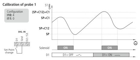
Parameter **CO** allows for correction of the temperature detected by probe 1; this is particularly useful when the probe cannot be located in the ideal place.
