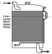
Figure 4: Atmospheric System
