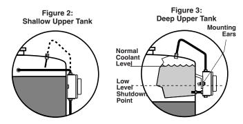
For a PRESSURIZED system the tip of the copper tube will be the shutdown level.
