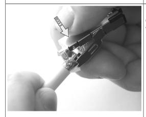
Close the terminal block. Make sure that the terminal block is fully closed.
