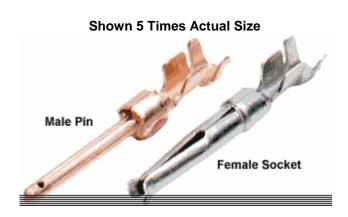
All pins and sockets can be easily wired using NEWPORT® thermocouple wire in either solid or stranded construction, 20 or 24 gage. Stranded wire is recommended so that electrical connections will have higher reliability. These precision Sub-D connectors are sold in sets of five, each package consisting of 5 male connector bodies and 5 female connector bodies. Sets are available in 9, 15, 25, 37 and 50-pin configurations.
