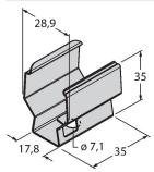
Snap bracket for mounting WLS28 work lights
