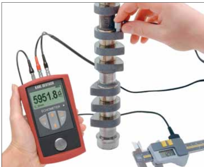
ECHOMETER 1076: Sound velocity measurement on a camshaft
