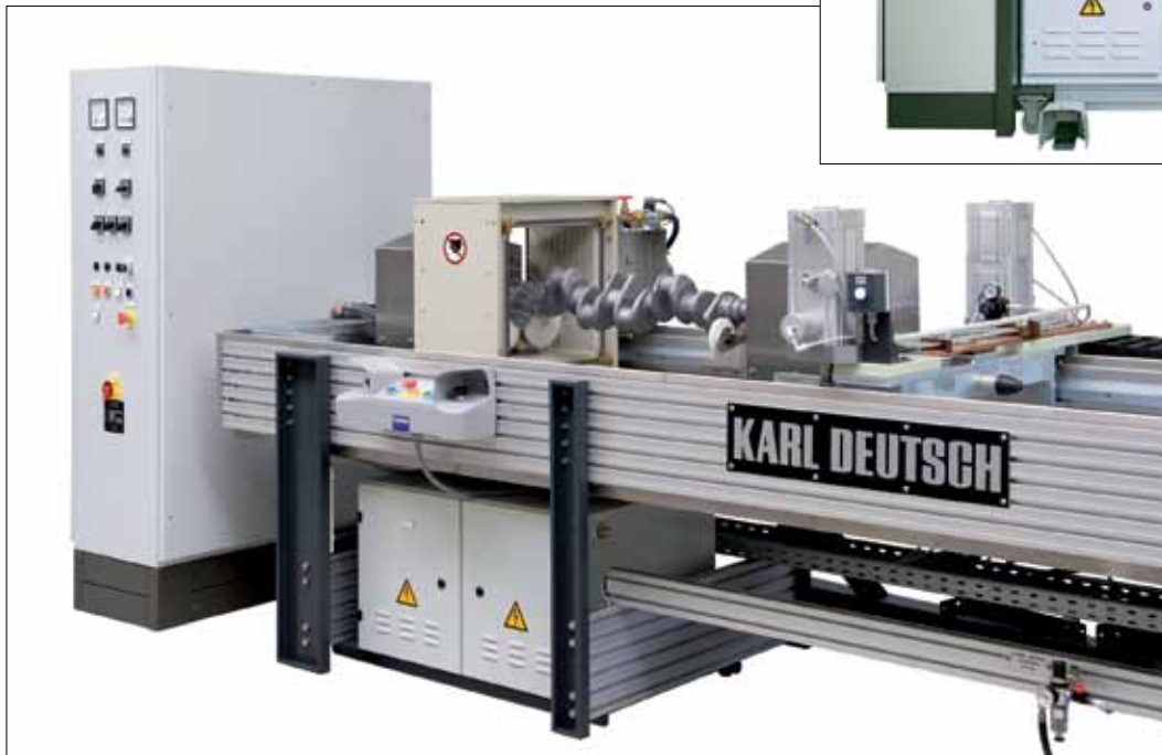
Test of a crankshaft with moving coil (DEUTROFLUX® UWS 2500)
