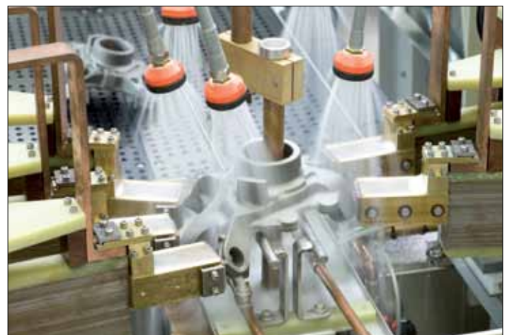
DEUTROMAT with 5 contacts and magnetization bar, universally adjustable
