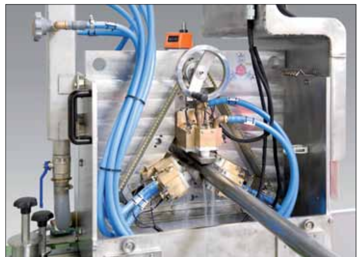
Testing system for bars with diameters up to 130 mm with 9 probes
