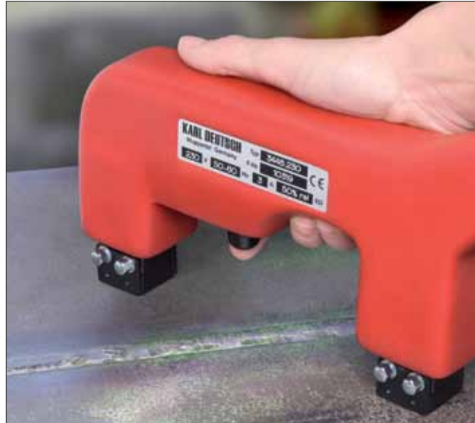
Handheld yoke for weld inspection (DEUTROPULS 3446)
