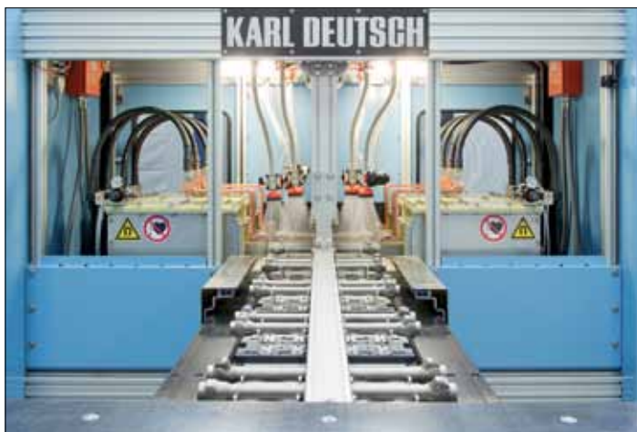
DEUTROMAT with chain conveyor, 8 components per cycle
