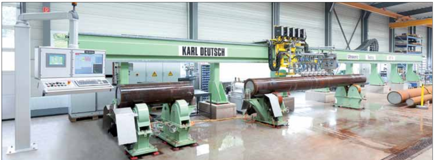
Testing portal for seamless tubes with 6 probe holders containing 30 probes
