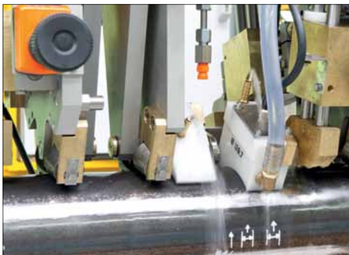
Phased array test system for welded pipes (ERW)
